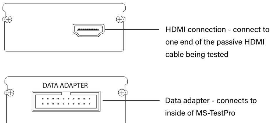
The Looper module is a remote-end module with RJ45 and HDMI ports that is used to create the loop at the other end for HCT testing (and DC Resistance when purchased with the optional DCR module). A Looper is supplied with any HCT or DCR module purchase.
