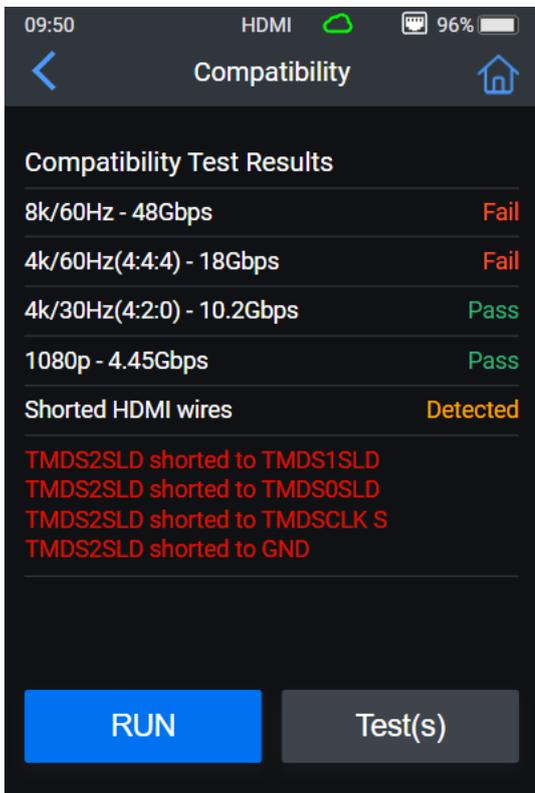
**8K/60Hz - 48Gbps:** testing the cable for its ability to carry 48Gbps to the Ultra High Speed classification for use with the HDMI2.1 chipset
