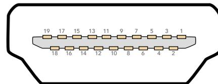
The TMDS (Transition-Minimised Differential Signaling) channels are used for the transfer of video, audio and clock signals which are all required to carry high-speed data.
