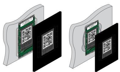
11 \*Optional\* To ensure the face plate stays in place, use the included face plate screw and thread it through the bottom of the face plate (an extra screw is included in case one is lost).
