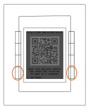
For easy network configuration, press and hold the bottom left & right buttons for 2 seconds. Once released, it will open an advanced options screen.
