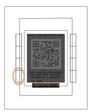
Modes can also be switched by pressing the bottom left hand button from the main screen.
