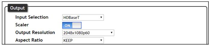
3. Select the resolution and timing for the output to scale to.
