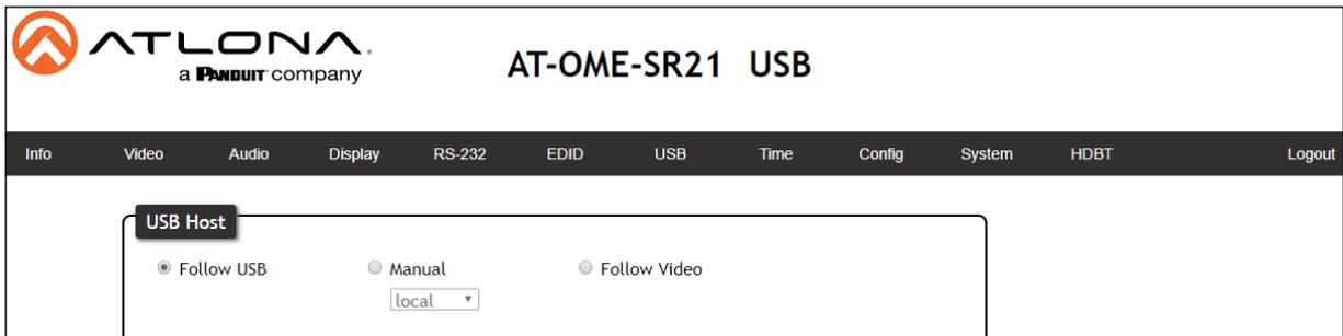
**Follow USB** - Assigns the USB devices to follow the most recently connected Host (e.g. Computer). If a new USB device is connected, then it will auto switch to that Host. If the current host is disconnected, it will fall back to the previously connected active device.
