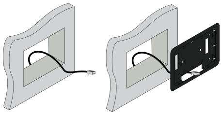
6. Press a screwdriver into the triangle metal flaps of the unit to secure the VTP-FMK into the wall. There are 8 triangles to press in, two on each side.
